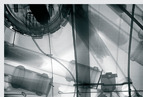
X-ray of drugs in pipes in fuel tank
