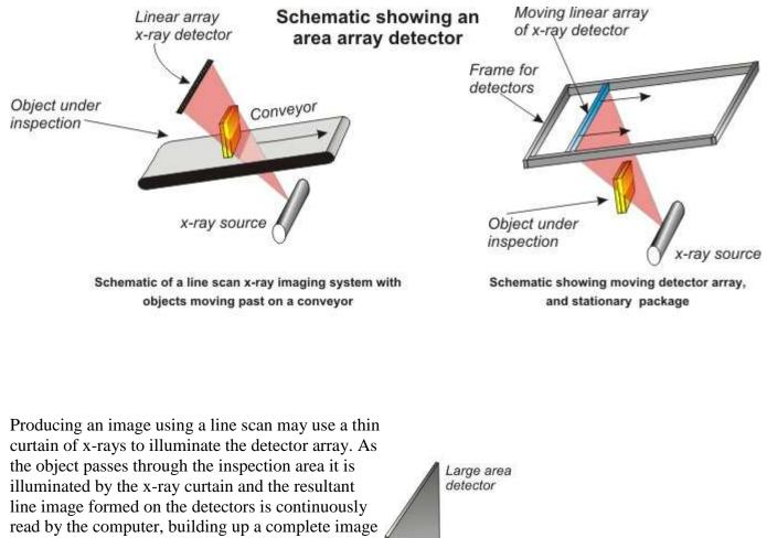
of the object line-by-line. This technique also reduces the x-ray exposure to the object being inspected by around 98%.
