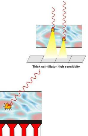
Scintillator bonded to detector
